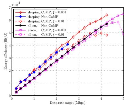
Fig. 4. EE versus data rate targets. Optimal cluster size,  $P_{sp} = 50$  W.
