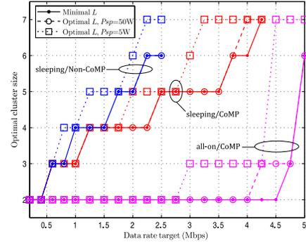
Fig. 3. Optimal cluster size ( $L + 1$ ) versus data rate targets,  $\xi = 0.001$ .
