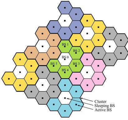
Fig. 1. An example of considered network model. Each cluster consists of 6 cells, where BS<sub>0</sub> is switched off and BS<sub>1</sub>-BS<sub>5</sub> serve all users in the cluster.
