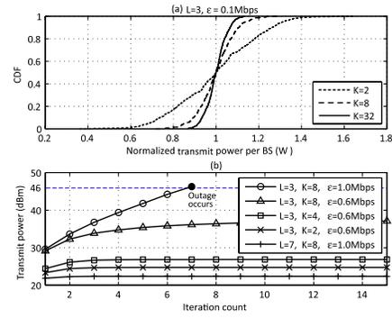
Fig. 2. CDF of normalized transmit power per BS,  $P_{\text{tx}}^{b,c}/\mathbb{E}\{P_{\text{tx}}^{b,c}\}$ , and convergence behavior of the proposed algorithm.
